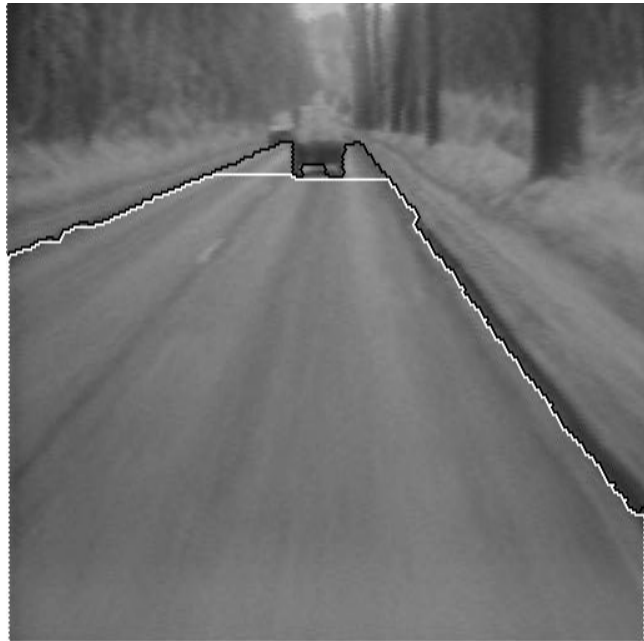
Figure 19: Obstacle-free zone. In black the edges of the road. In white, zone without obstacles in front of the car.
