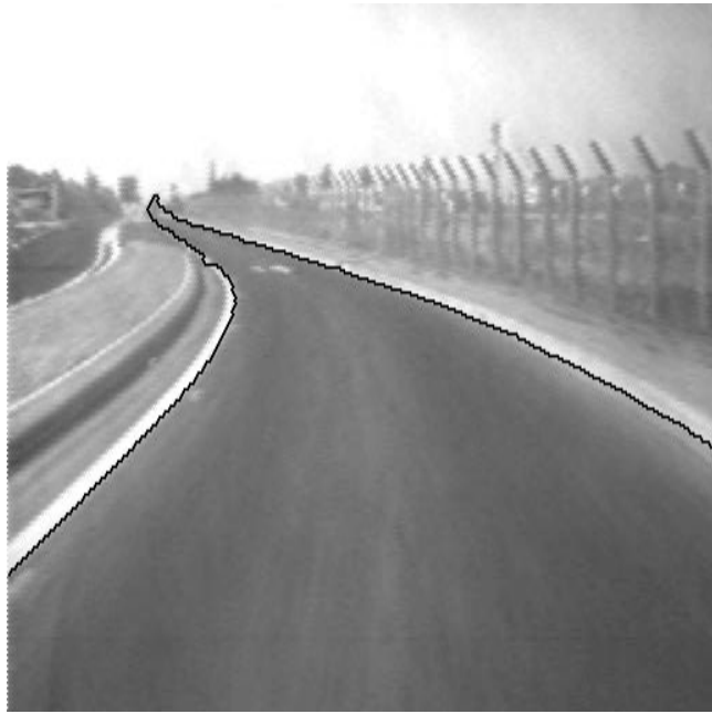
Figure 27: Curved road segmentation
