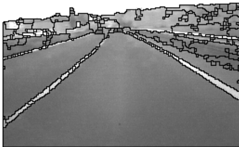
Figure 3: Watershed of the gradient of the filtered image
