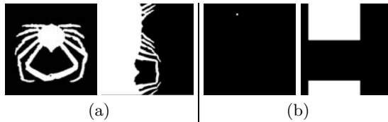
Fig. 1. (a) Example of conversion (x, y) \rightarrow (\rho, \omega) ( (x_c, y_c) corresponds to the body center of the crab). (b) Dilatation of one point by a square in log-pol coordinates.
