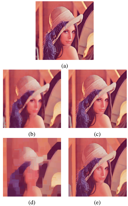
Fig. 1. Example of color levelings using the lexicographic order I - RGB_{\alpha=10} on Lenna image: (a) Reference image, \mathbf{f} . (b) Marker (ASF of size 5), \mathbf{m}_1 . (c) Leveled image, \Lambda(\mathbf{f}, \mathbf{m}_1) . (d) Marker (ASF of size 15), \mathbf{m}_2 . (e) Leveled image, \Lambda(\mathbf{f}, \mathbf{m}_2) .
